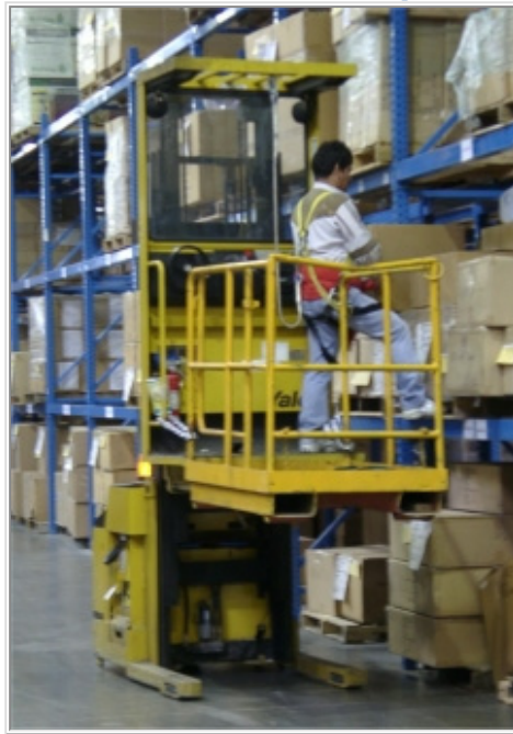
Above: Single Case Retrieval using a Man Up Platform Truck
