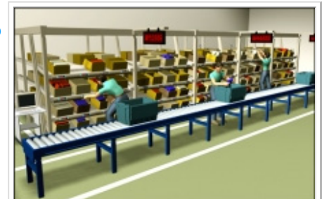
SKUs on Conveyor put to Orders in Flow Rack by Lights
