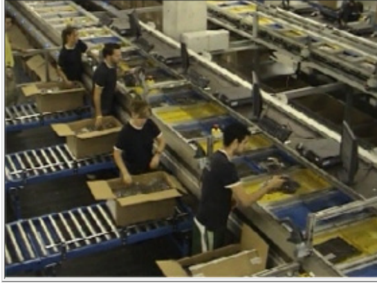
Above: Sorter Induction Stations for a Bomb Bay Style Sorter - Euorsort
